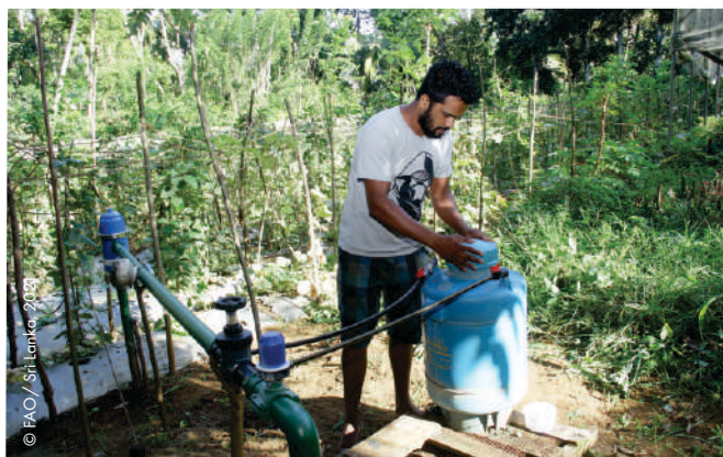
The workings of fertigation through drip irrigation
